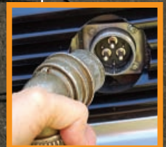
A large plug allows electricity to move from the car to the power lines and back.
